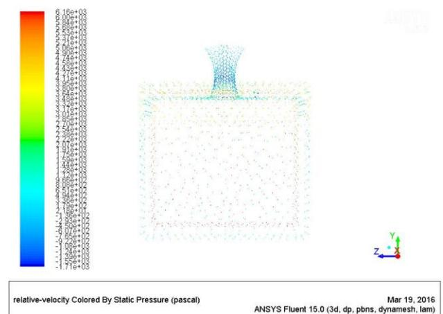
Fig :5 Relative Velocity Colored by Static Pressure
