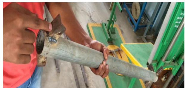
Fig.8. Welded flanges with provision for bolting
