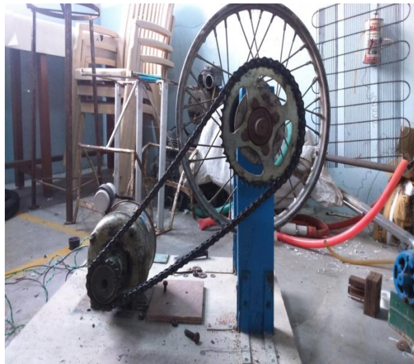
Fig.5. Chain drive unit with 0.5HP motor
