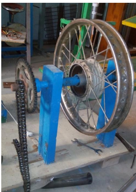
Fig.6. Motorcycle rim used as Rope drum
