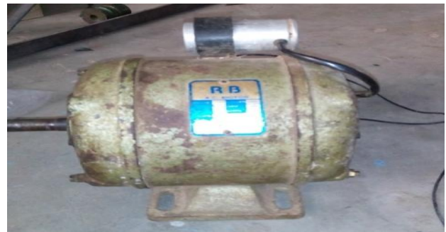
Fig.1. 0.5HP AC motor used in hoisting device
