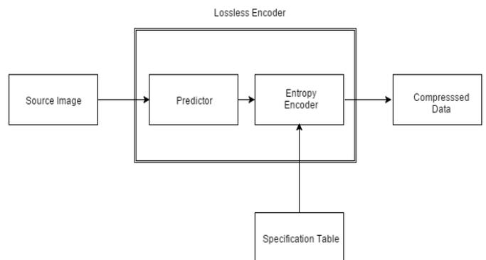
Fig-4: Lossless Compression
