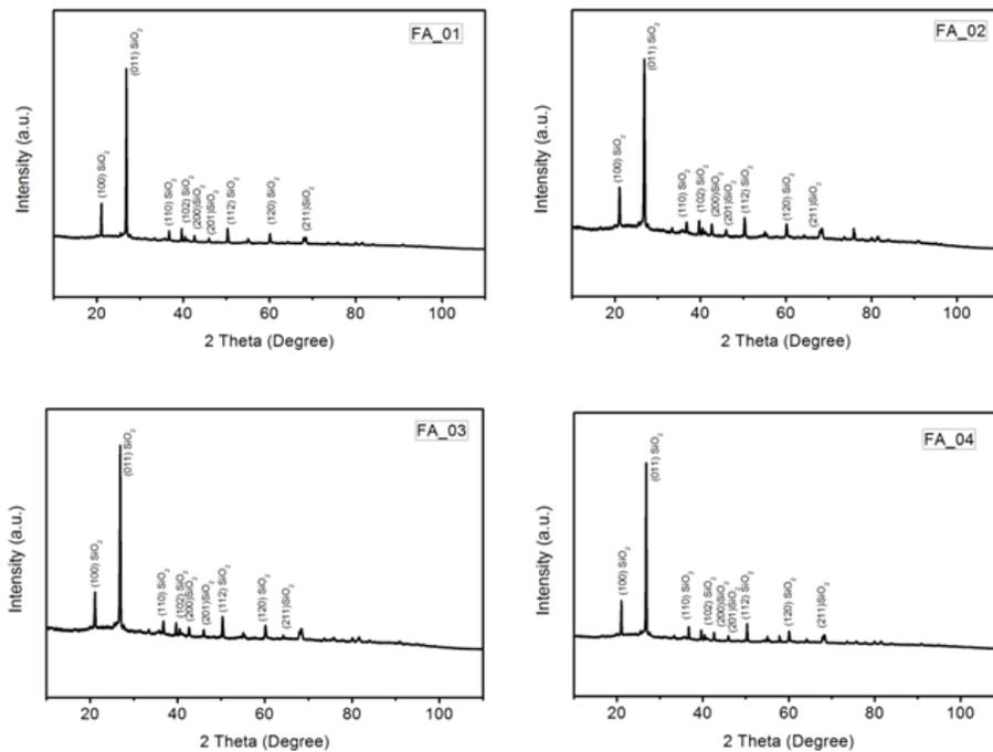
Figure 3: X-ray diffraction pattern (XRD) of Fly ash
