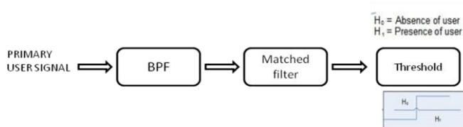
Fig 2. Matched filter detection
