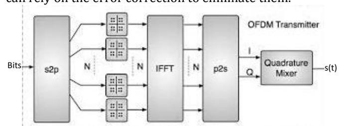
Fig 1. Block diagram of OFDM
