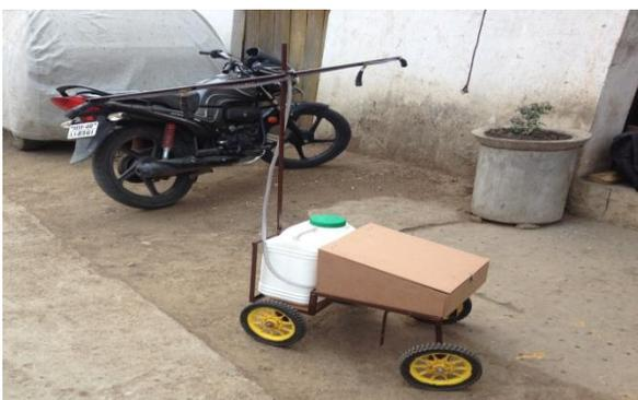
Image 1 : Actual Photo of Automatic Pesticides Spraying Machine
