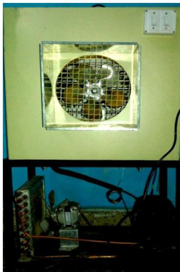
**Fig.3.2 VCRS Based Cooler.**
