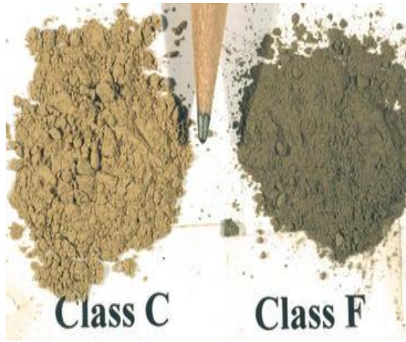
Fig: 03 An original image of class F and class C fly ash [31]
