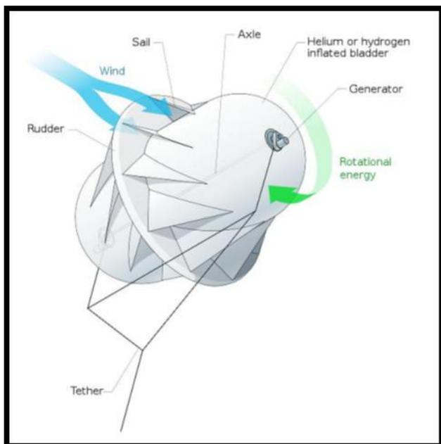
Fig -2: Construction of a FEG
