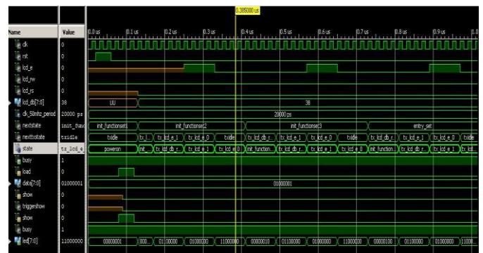
Fig-4: Simulation Output of 8x10 Encoder with Ripple Counter
