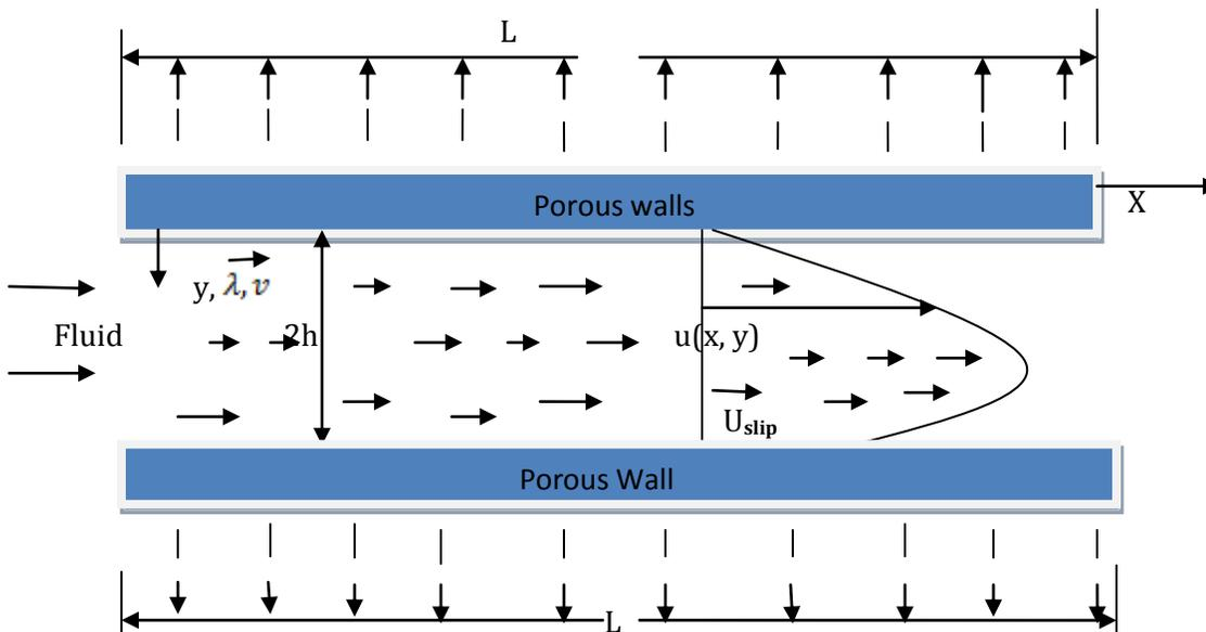
Fig. 1. The coordinate system used in the solution of the two dimensional steady State flow of Non-Newtonian fluid.
