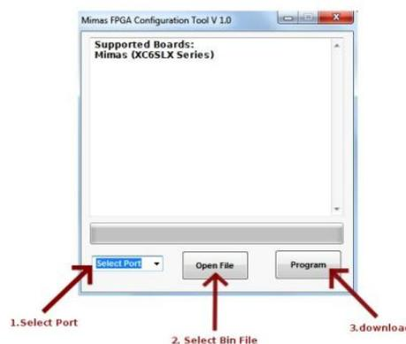
[2]The above snapshot shows configuring Mimas. Open Mimas Configuration Tool. Select the port no.
