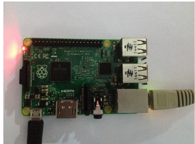
Fig -9: Hardware implementation on Raspberry Pi
