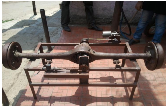
Fig -1: working of "Automobile Reverse Locking Differential Mechanism".
