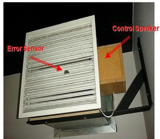
**Fig 3. Error microphone and loudspeaker mounted in duct.**
