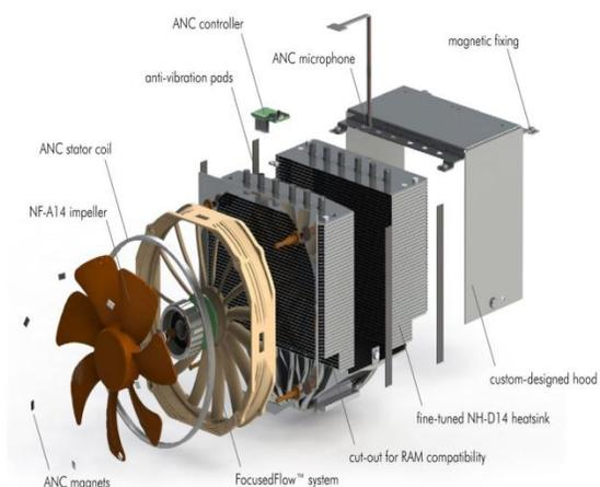
**Fig 4: Active Noise Cancellation Installation Device**
