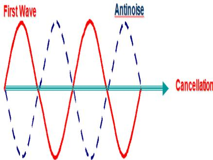
**Figure 1. The mechanism of active noise cancellation control.**
