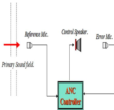
**Figure 2. Basic structure of a feed forward active noise control system**
