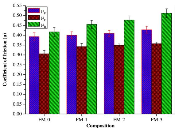
Fig -2: Friction performance of the brake friction materials:  $\mu_p$ ,  $\mu_f$  and  $\mu_r$
