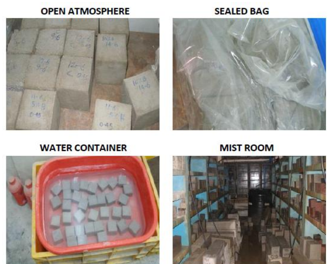
Fig -4: Different curing conditions
