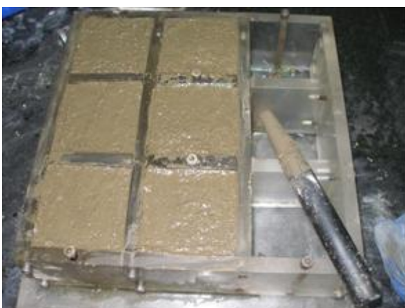
Fig -3: Moulds of dimension 70 x70 x 70 mm filled with mortar using tamping rod
