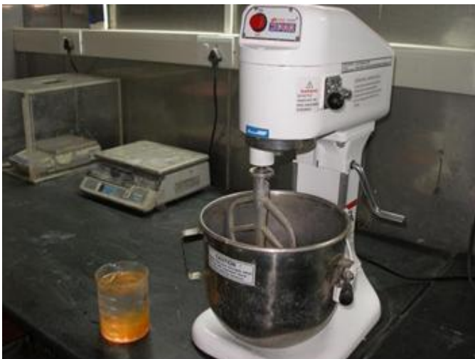
Fig -2: Mortar mixer and beaker filled with water and SAP beads
