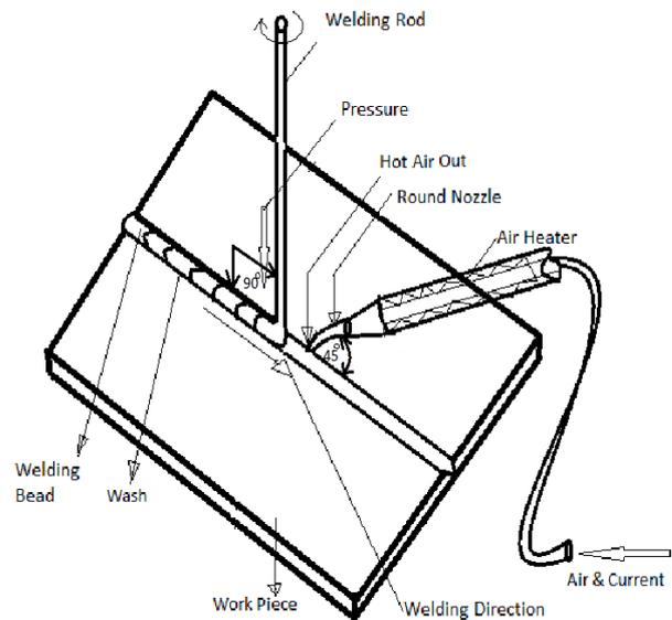
**Fig. 4** systematics of hot gas welding [3, 1].
