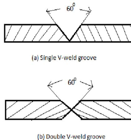
**Fig 2** geometries of weld groove. (a) Single V-weld grooves. (b) Double V- weld groove [7].
