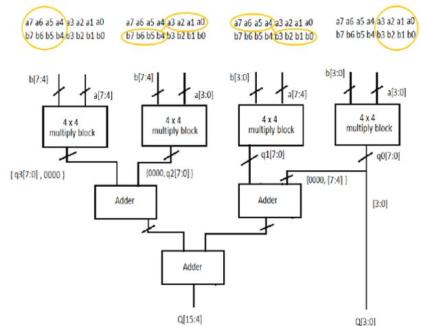
Figure 5.1 Structure of MODIFIED BOOTH MULTIPLIER
