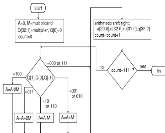
Figure 4.1 Structure of MODIFIED BOOTH MULTIPLIER
