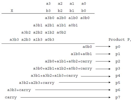
Figure 3.1 Structure of BAUGH WOOLEY multiplication
