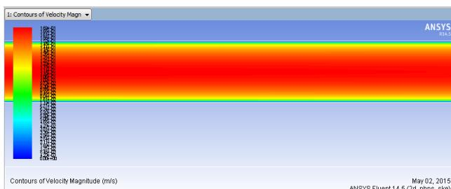
**Fig. 6** Contour Plot of Velocity Magnitude of Smooth Pipe
