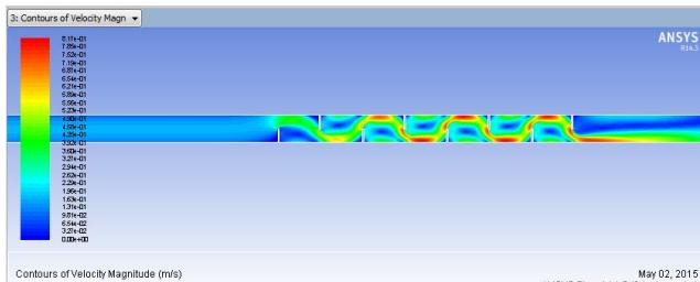
**Fig. 7** Contour Plot of Velocity Magnitude of Segmented baffles Pipe
