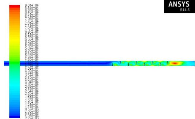
Contours of Turbulent Intensity (%)
