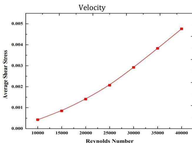
**Fig. 5** Variation of Shear Stress with varying Reynolds Number
