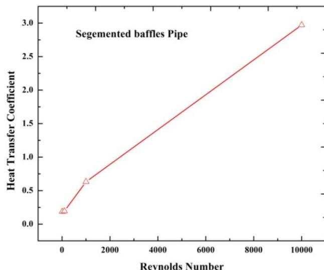
**Fig. 19** Variation of Heat Transfer Coefficient with respect to Reynolds Number
