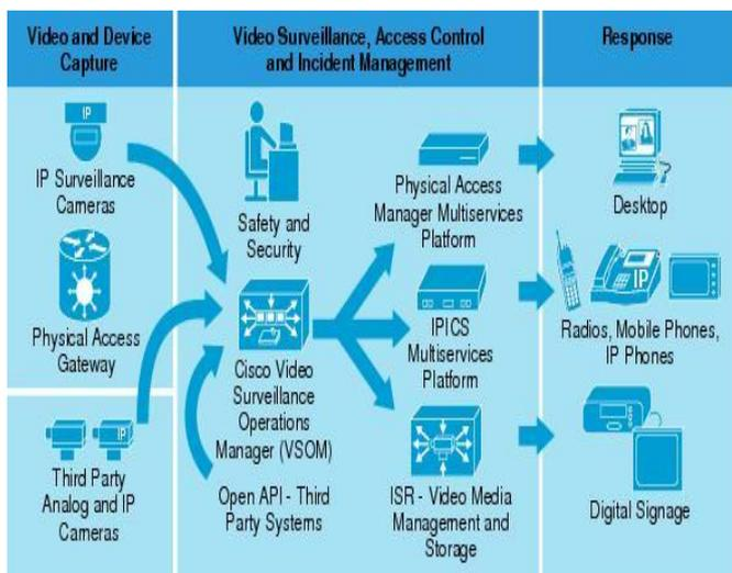
Fig -1: Architecture of video surveillance system
