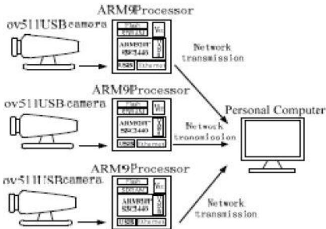
Fig -2: Structure of video capturing system
