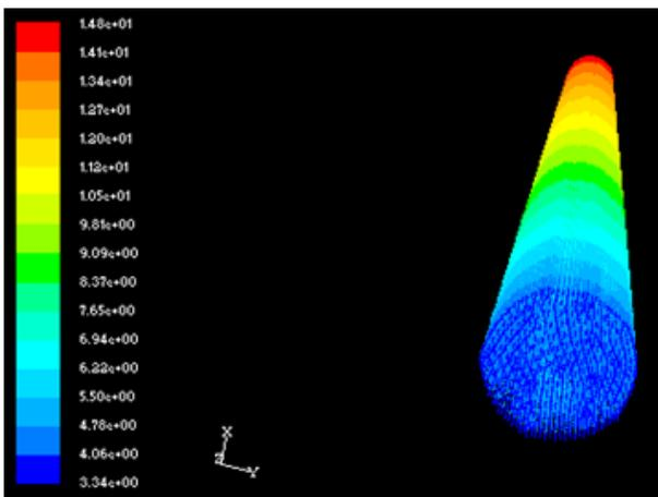
Fig-2: Catalyst velocity along the riser height
