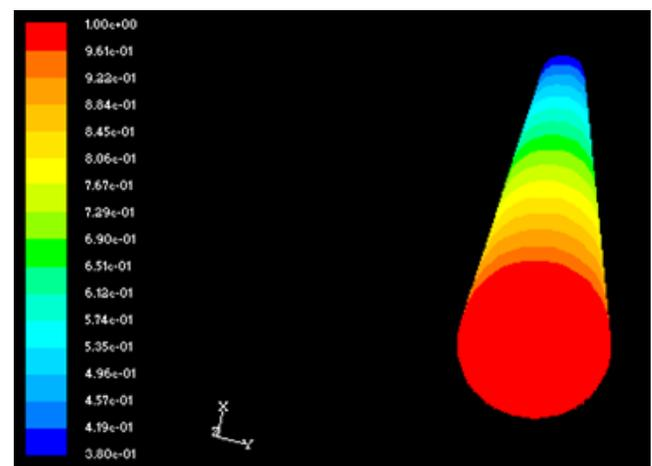
Fig-5: Gas-oil mass fraction along the riser height
