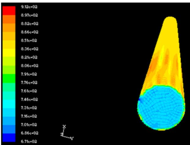
Fig-3: Gas phase temperature along the riser height
