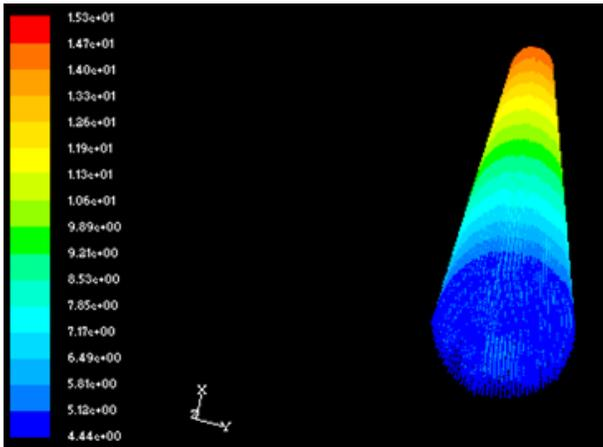
Fig-1: Gas phase velocity along the riser height
