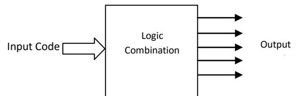
**Fig: Conceptual Diagram of Decoder**
