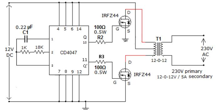
Fig -3: Circuit diagram of DC to AC Inverter
