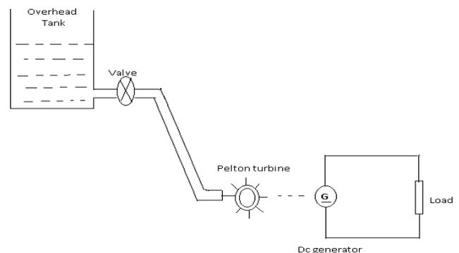
Fig -1: Micro Hydro Turbine System
