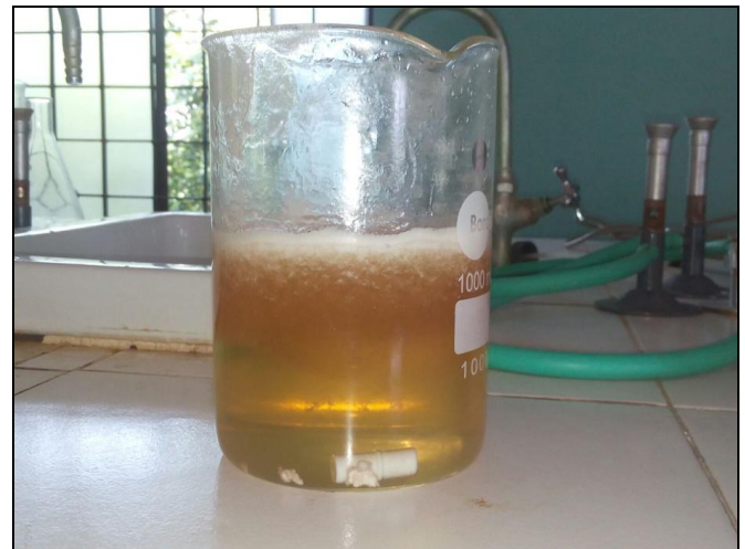
Fig -2.1: Three layer formation of biodiesel at bottom, ethanol at middle and glycerin at top.
