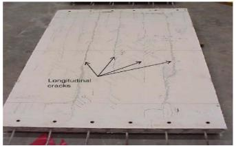
**Fig.4:** Typical Longitudinal shear failure
