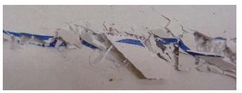
Fig.8: Longitudinal cracks
