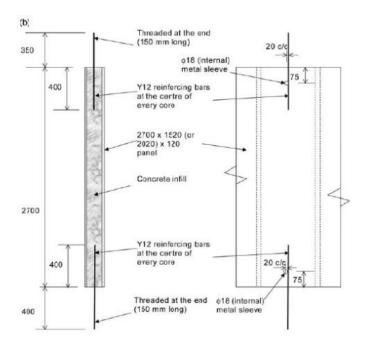
Fig.6 (b): Specimen with starter bars
