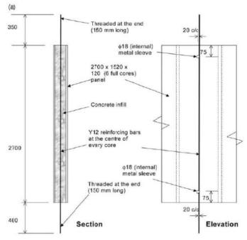
Fig.6 (a): Specimen with full length bars
