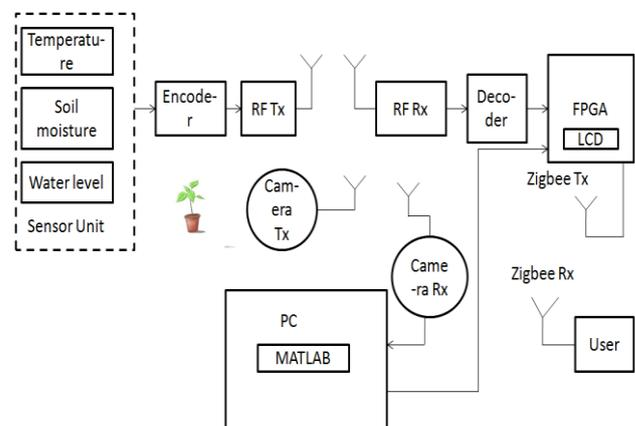
Fig-1: Block diagram of plant monitoring system design
