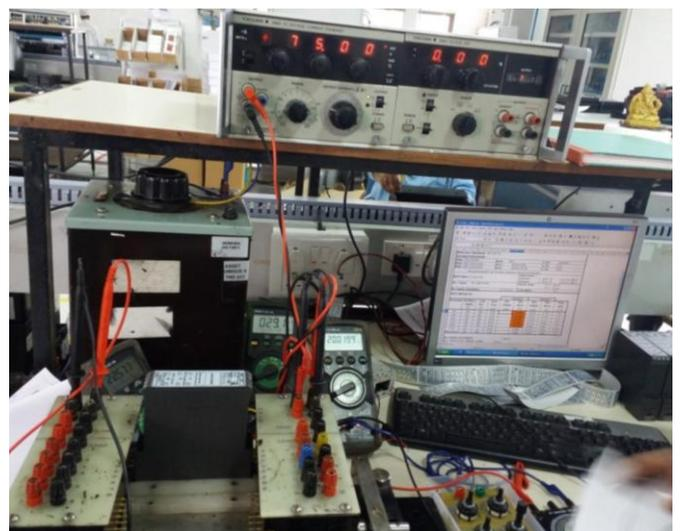
**Figure-2** The closed loop system for transducer using YOKOGAWA Calibrator
