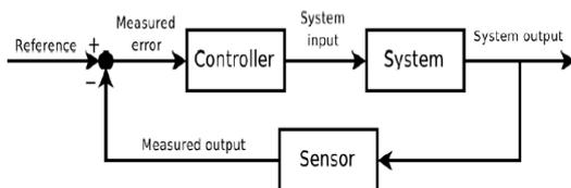
**Figure-1** Basic Feedback Loop System
