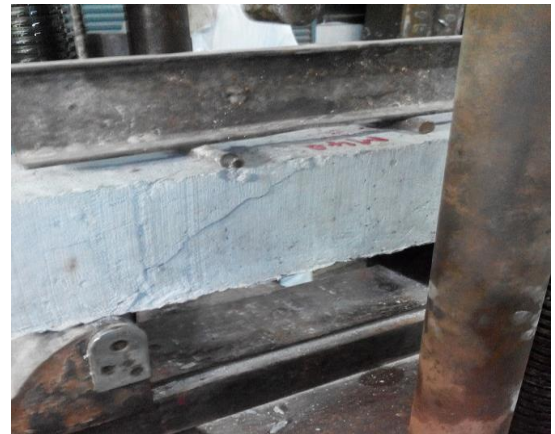
Crack Behavior of Specimen After Application of tensile load for 28 days
