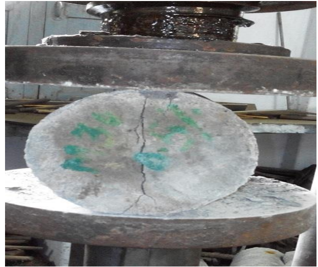
Crack Behavior of Specimen After Application of tensile load for 28 days
