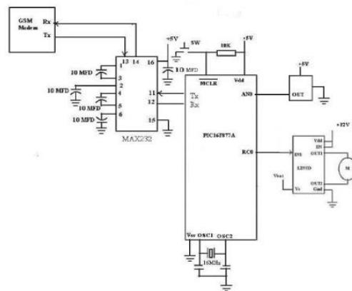
*In the above diagram, port A is configured for analog inputs. AN0 is connected to the temperature sensor, pin RCO is responsible for the connection of the motor. MAX232 converts 12V DC into 5V DC and vice versa is connected to port C. The transmitter and receiver is connected to 11<sup>th</sup> and 12<sup>th</sup> pin of MAX232.*
