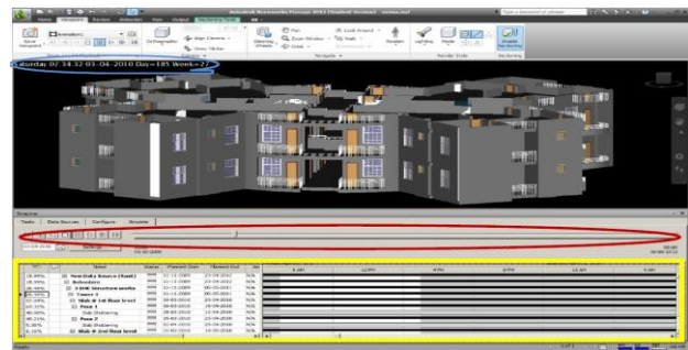
Figure 3.2 4D MODEL showing the progress of the building at 27th week
