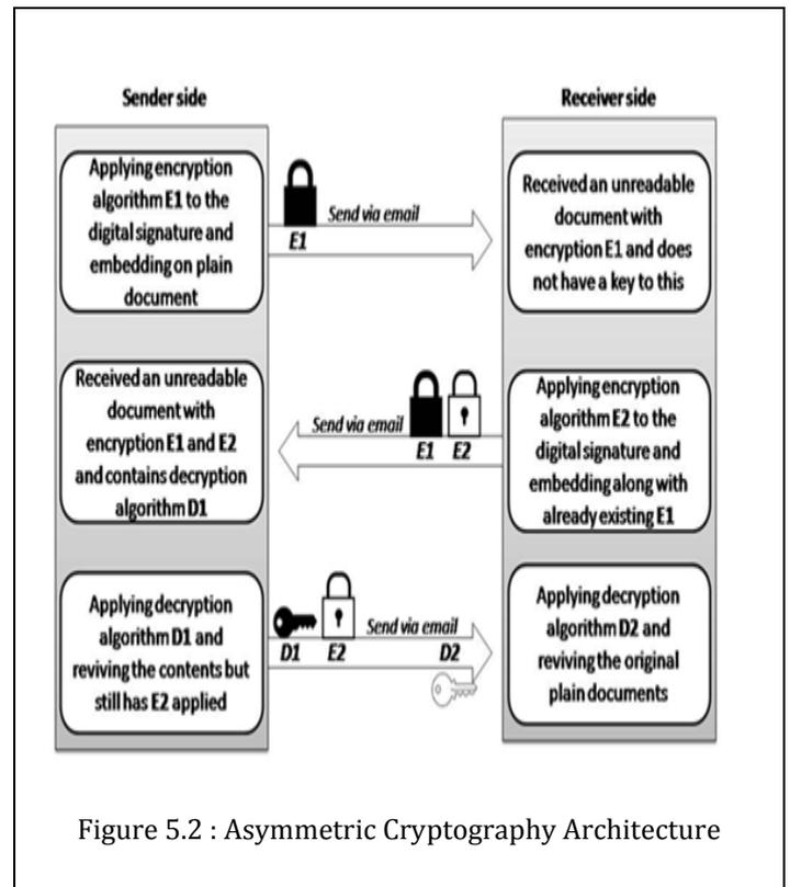
Figure 5.2 : Asymmetric Cryptography Architecture
