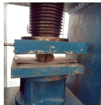
Fig. 5 Split tensile strength test
