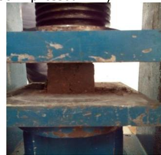
Fig. 4 Compressive strength test
