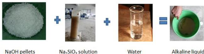
Fig. 2 Preparation of alkaline solution
