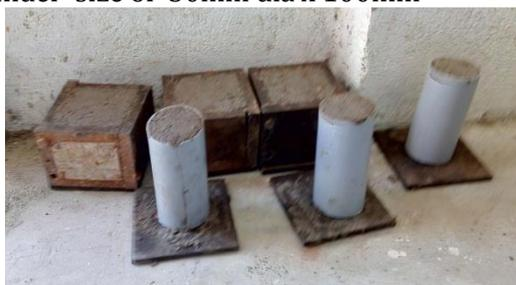
Fig. 3 Specimens casted for testing
