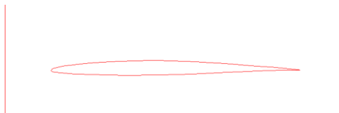
Fig. 9.0 Airfoil of first prototype NACA 64A206
