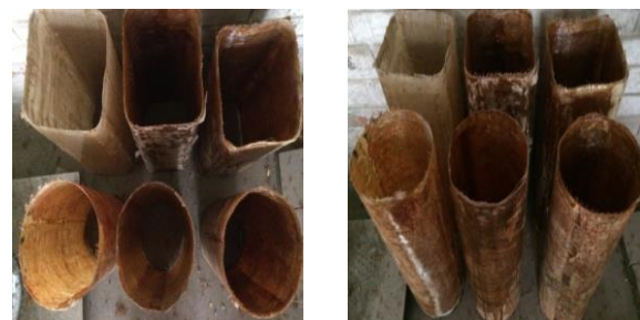
Fig-2: Photograph of FRP Tubes
