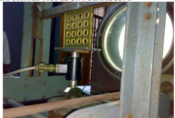
Fig. 3.1 Experimental setup of perforated model on polariscope
