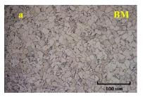
**Figure 17.** Microstructures of P11 steel base metal after PWHT at 850°C.
