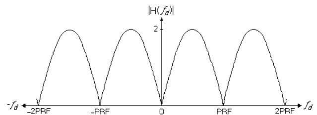
Fig.-2: Frequency Response of MTI Filter.
