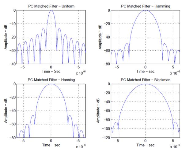
Fig-5: Windowing Function
