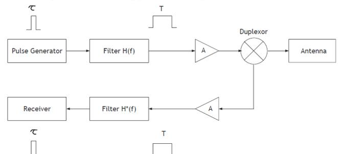
Fig-1: Pulse Compression signal generation
