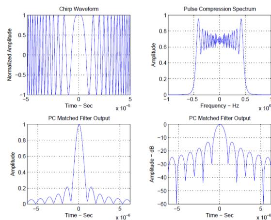
Fig-4: Pulse Compression Matched Filter Output
