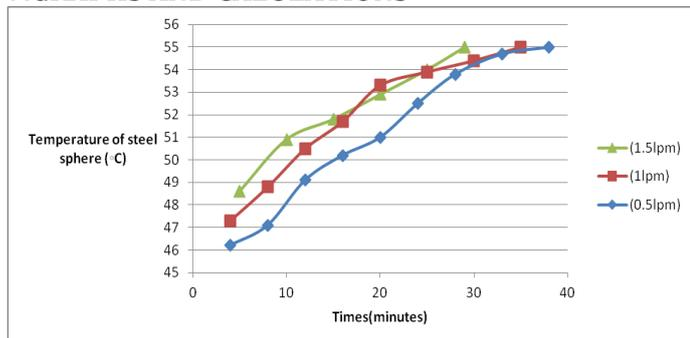
Figure 1. Temperature of steel sphere v/s time at different flow rate with water
