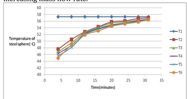
Figure 4. Variation of temperature v/s time at different segment of bed with Al<sub>2</sub>O<sub>3</sub>/water (0.1 % concentration)
