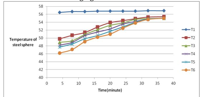
Figure 2. Temperature v/s time at different section of packed bed
