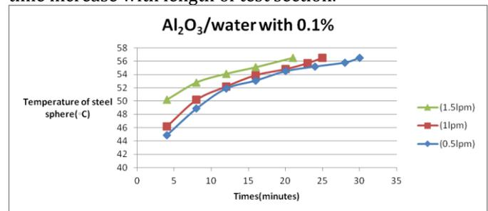
Figure 3. Temperature of steel sphere v/s time at different flow rate with Al<sub>2</sub>O<sub>3</sub> with .1% concentration.
