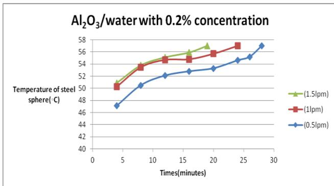
Figure 5. Temperature of steel sphere v/s time at different mass flow rate with Al<sub>2</sub>O<sub>3</sub>/water (0.2% concentration)
