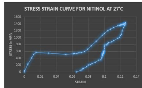
Fig 4: Strain Curve for Nitinol at 27 °C
