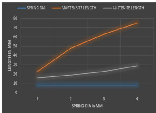
Fig 12: Plot of Spring Diameter V/S Length
