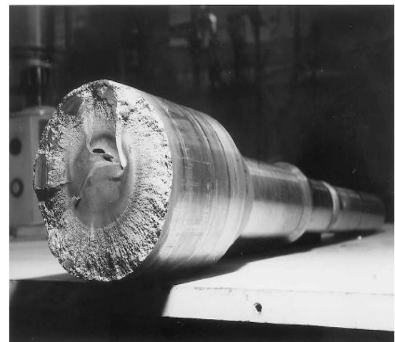
Fig- 4: Photographs of the failed shaft [4]
