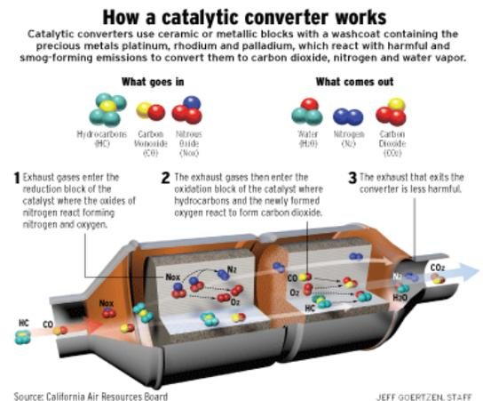
**Fig -1** Typical Three-way catalytic converter
