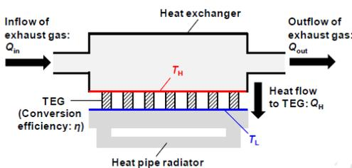
Fig -4 Thermo electric generator
