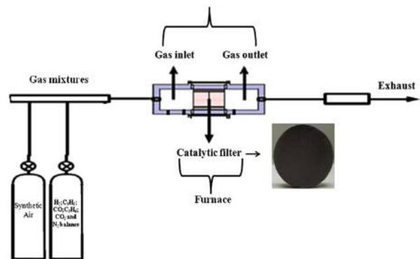
Fig -3 Schematic drawing of the experimental setup used to evaluate the Catalytic efficiency
