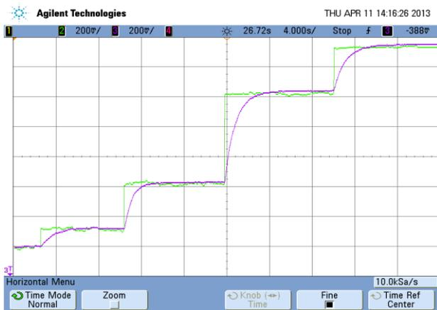
Figure 9 Dynamic speed waveform of PI-ILC-SVPWM
