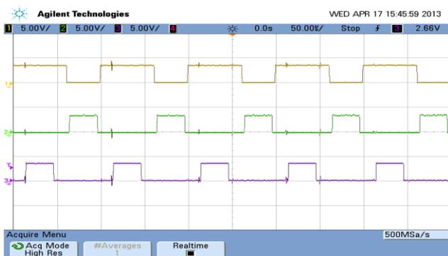
Figure 10 Gate pulses waveform for phases G1,G3,G5
