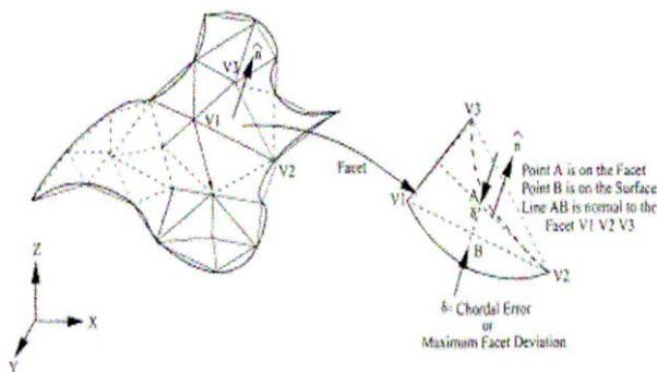
**Figure 1: The tessellation of a typical surface of CAD model [2](after pandey et al. 2003b)**
