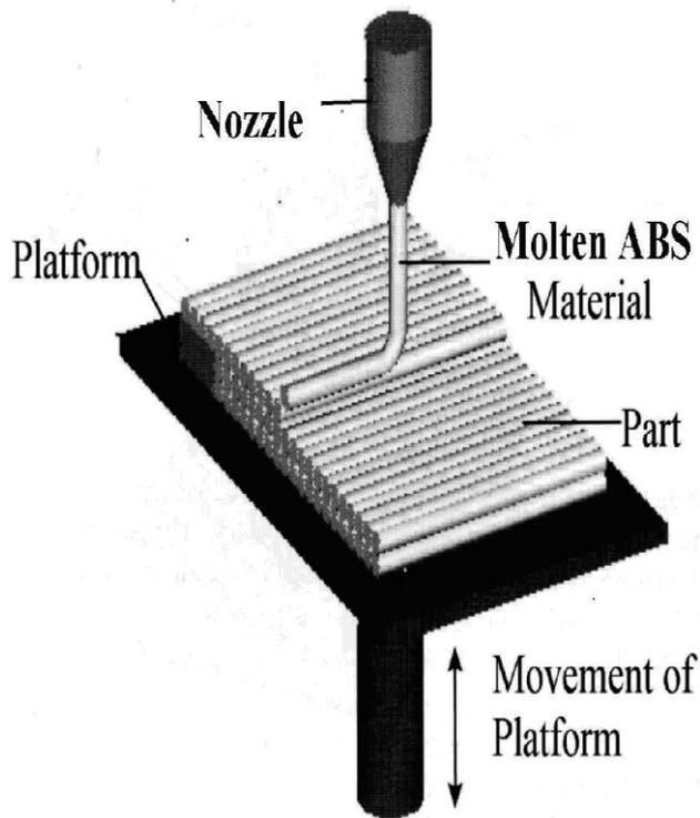
**FIGURE 4: FUSED DEPOSITION MODELLING PROCESS[3] (after pham and demov,2001)**
