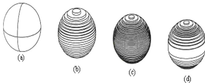
**Figure 10: Slicing of a ball, (a) No slicing (b) Thick slicing (c) This slicing (d) Adaptive slicing [3] (after Pham and Demov, 2001)**
