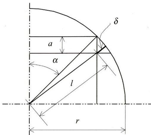
(b) Error due to replacement of arcs with stair-steps, cusp height [3] (after pham and Demov, 2001)
