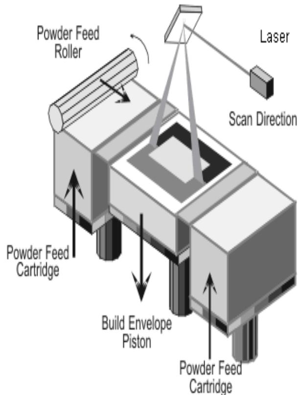
Figure 3: Selective Laser Sintering System
