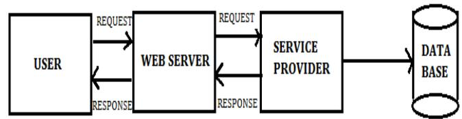
Above diagram shows that the Architecture of E-service Provider. It contain user, webserver, service Provider and database. Firstly user send the request to webserver then webserver gives a response to the user according to their request. Then webserver sends the request to service provider then service provider sends the response to webserver. At last service provider store all data in database.
