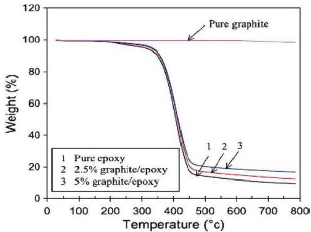
Fig 1: TGA curve of Epoxy GNP composite
