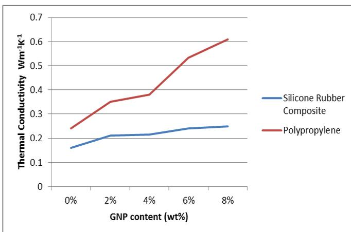
Fig 4 : Comparison of thermal conductivity of silicone rubber and polypropylene
