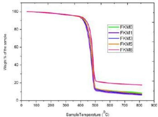
Fig 2: TGA curve FKM-GNP composite.
