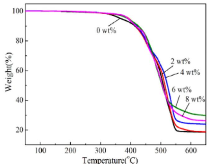
Fig 3 :TGA curve of Silicone GNP composite.
