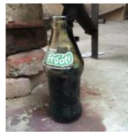
**Fig-12:** Oil obtained from PVC Pipes
