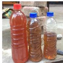
**Fig-8:** Oil obtained from injection moulding Grade 5
