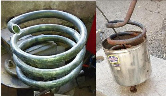
Fig -4: Heat Exchanger
