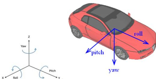
Fig -2: the orientation of tri-axis
