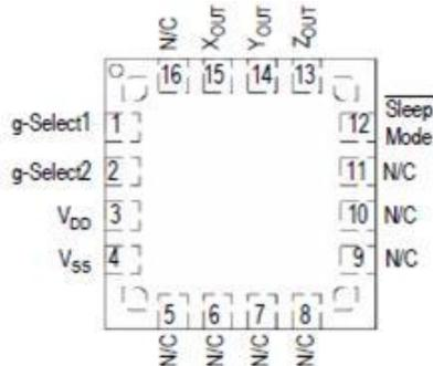
Fig -1: Pin Diagram of MMA7260QT
