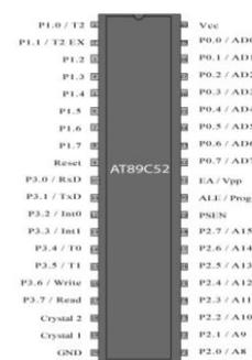
Fig -3: pin diagram of AT89C52 microcontroller
