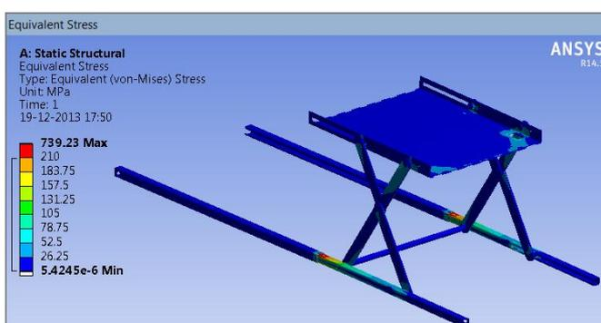
Fig. 8. Equivalent Stress
