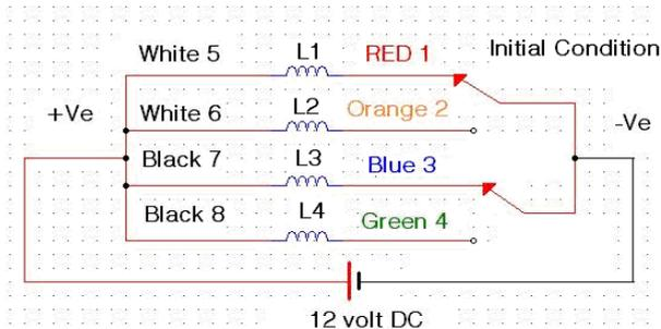
Figure: 8.1 Stepper motor winding arrangement
