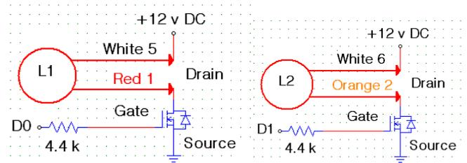
Figure: 8.2 (a) MOSFET ckt -I      Figure: 8.3 (b) MOSFET ckt - II
